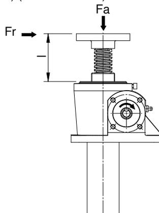
7. Check allowable side force  $F_r$  at the spindle according to table on page 29. For BD66,  $F_a=30 \text{ kN}$  and stroke 500 mm
